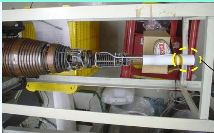
Sample cell made of PET tube ( $2.5\text{cm}^3$ )
