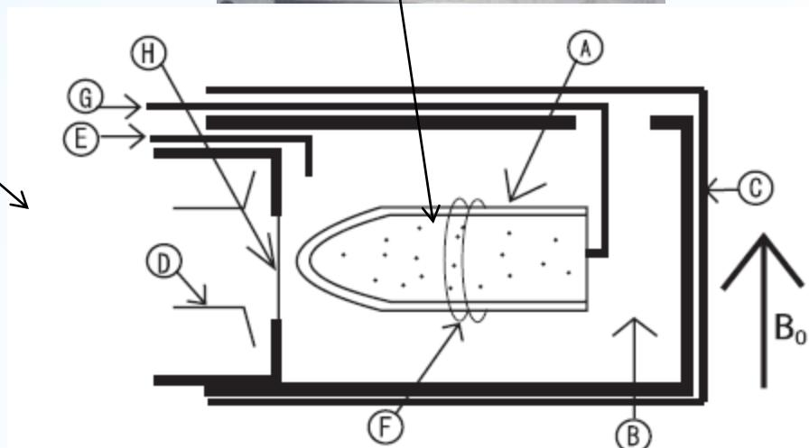
FIG. 1: Simplified diagram of the experimental setup showing A: the experimental cell; B: the  $^4\text{He}$  bath made of teflon; C: the copper wall to form a microwave cavity; D: a microwave guide(R-band) providing a microwave through the mylar window(H); E: a liquid  $^4\text{He}$  inlet; F: a 2-turn NMR coil, and G; a  $^3\text{He}$  inlet.
