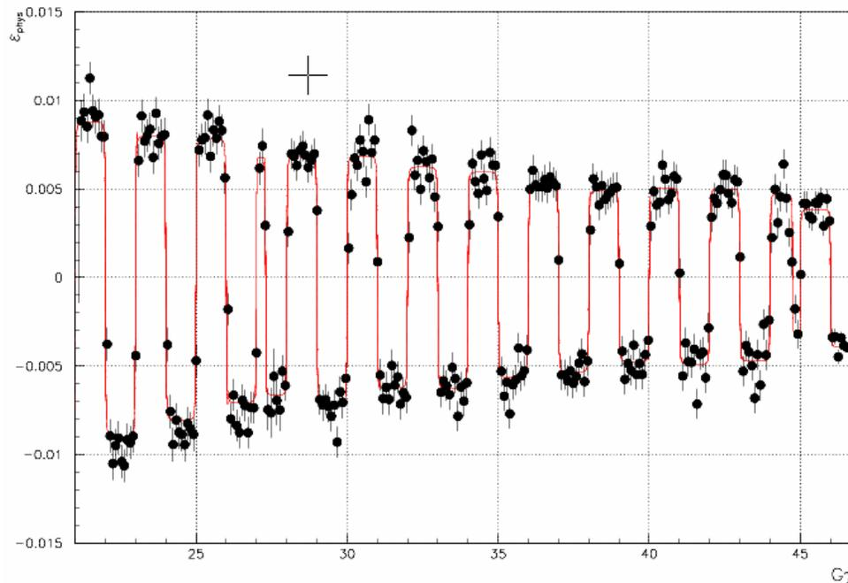
full spin flip at all imperfection and strong intrinsic resonances using partial Siberian snake and rf dipole at AGS
